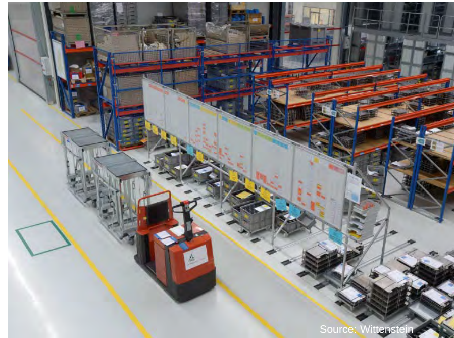
Electric train for material supply
